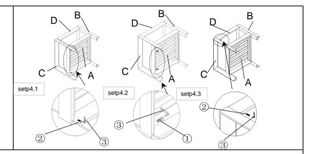
Step4.1:Attach Seat(A) and Backrest (D)to Right Armrest(C) using Bolts(2) with Allen Key(3) as shown above.
