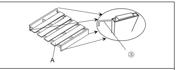
Open the carton and place all the parts onto a clean, non-marring surface. Take out the silders in the four ends of the Seat(A) using Allen Key(③).
