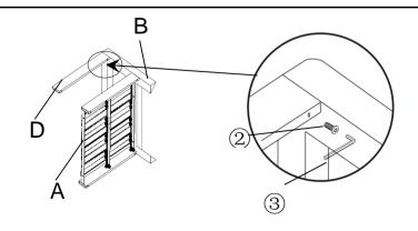
Attach Backrest(D) to Left Armrest(B) using Bolts(2) with Allen Key(3) as shown above. Do not fully tighten the Bolts.
