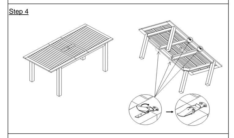
Lock the Metal Fasteners under the Table Top to lock the Expansion Board of Table Top(A) into place as shown in the above picture.
