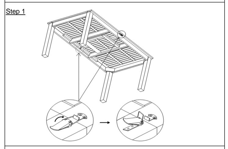
Unlock the Metal Fasteners.
