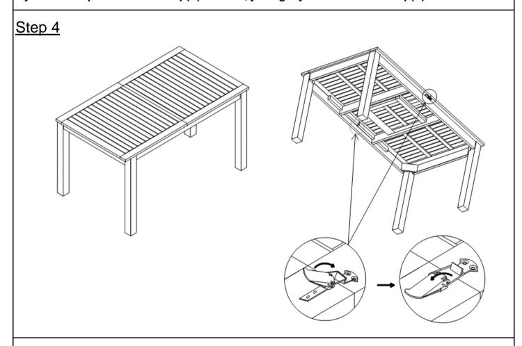
Lock the Metal Fasteners under the Table Top(A) into place as shown in the above picture. Your Table is retracted and is now ready for use.
