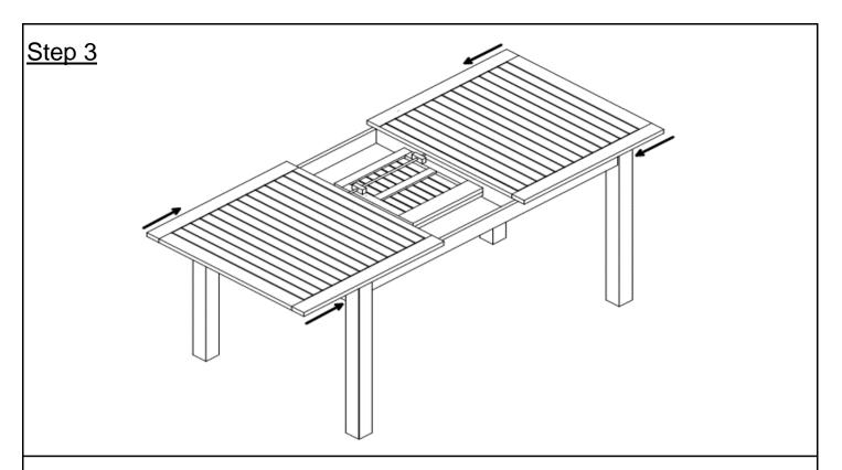
Push the Table Top(A) inwards until both wings of the Table Top(A) align.
