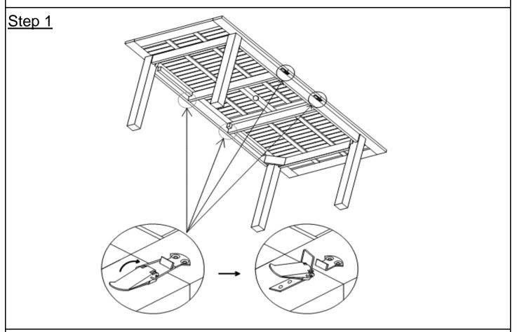
Unlock the Metal Fasteners.
