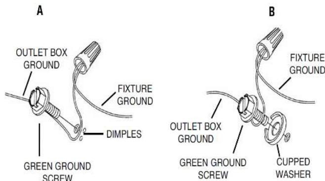
**Connect wires according to below chart**
