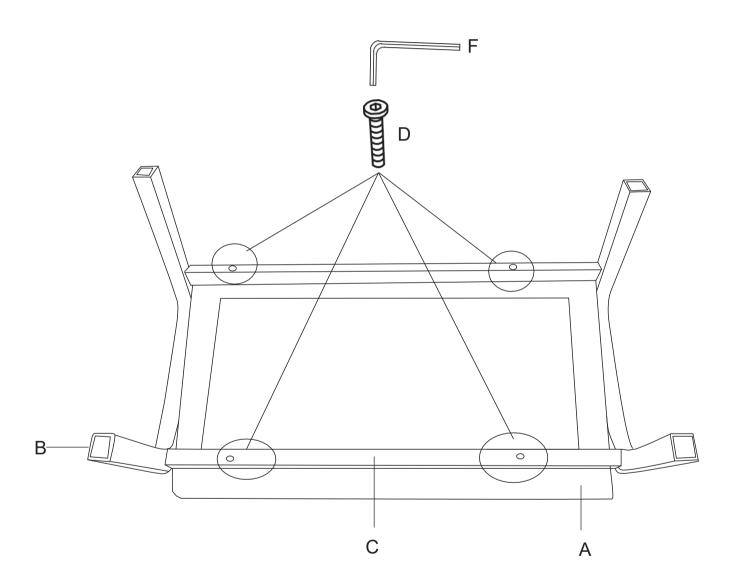
**STEP 3** Please 100% tighten all Allen Bolts (D,E) completely by using Allen Wrench (F).
