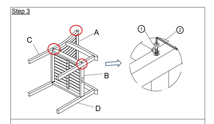
With assistance from an adult partner, turn the Chair Frame over onto the other side. Attach First Leg Panel(C) to Backrest Panel(A), and Seat Panel(B) using Screws( $\widehat{1}$ ) with Allen Key( $\widehat{2}$ ).
