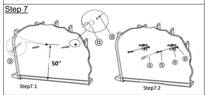
**7.1)** Use Power Drill(9) Drill two mounting positions on wall at same height, bury Plastic Anchor(10) into the mounting position with a Hammer(1) (No priovide).
