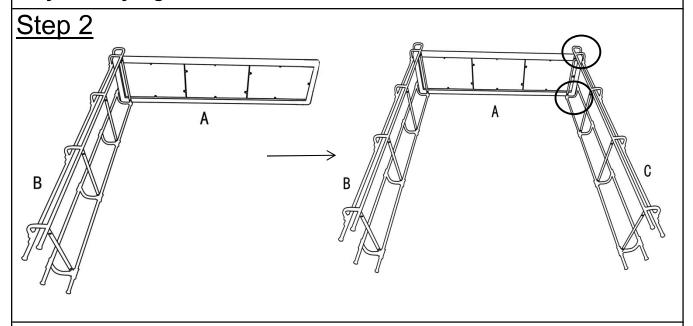
Attach Wooden Shelf(A) to Right Leg Frame(C) using Bolt(③) with Allen Key(④).
