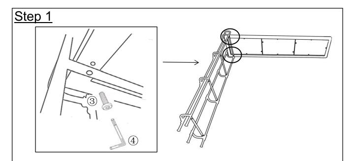
Open the carton and place all parts onto a clean, non-marring surface. Place the Left Leg Frame(B) on it's side as shown.
