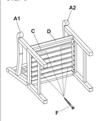
Lay down the chair and secure the seat using 1" screws (F) as shown. Tighten using screwdriver.
