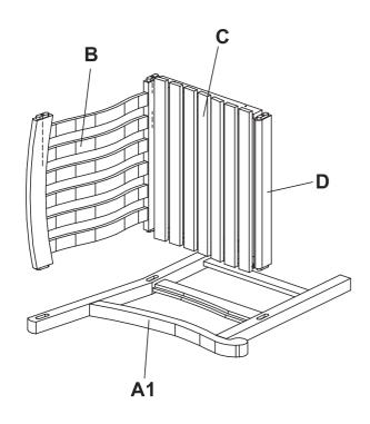
Attach back support (B),apron (D) and seat (C) into right side frame (A1).
