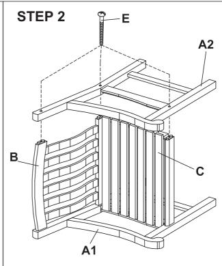
Attach left side frame (A2) to the assembly from step 1 using 1 1/2" bolts (E).
