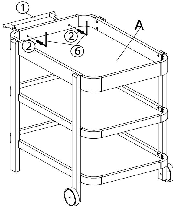
To affix the Handle (①) to the Upper Tray (A) , align the bolt mounting position of the Handle to the mounting positions at the Upper Tray.
