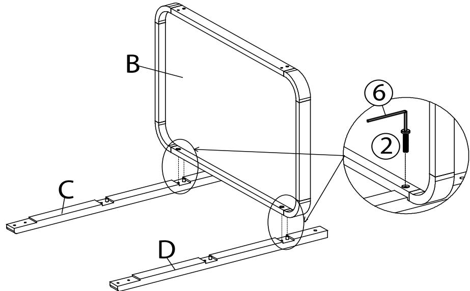
Place the Long Leg(C), Short Leg (D) facedown as shown in picture above.
