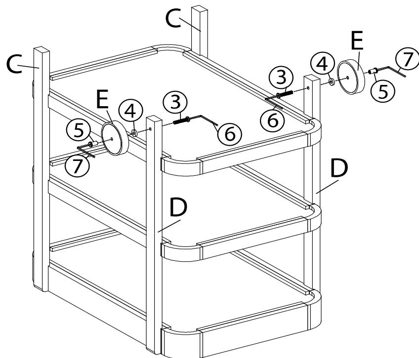
With the assistance from your partner, turn up side down the pre-assembled on step 6. Secure the Wheels (E) to Short Leg(D) by using Bolt (3), Washer (4), Sleeve Nut(5) with Allen Key (7) and Allen Key (6) as shown above.
