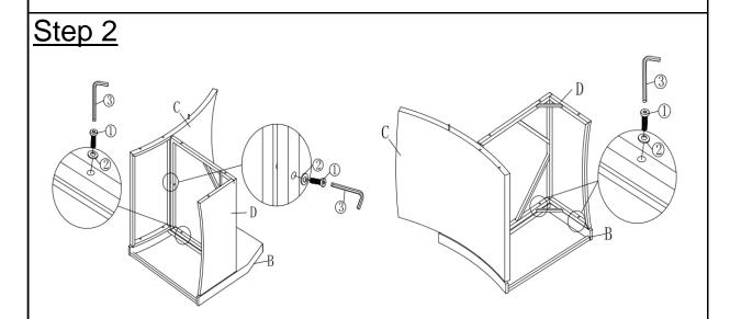
Attach Seat (D) between the Right Armrest (B) and Sofa Back (C) using Bolts (1) and Washers (2) with Allen Key (3) as shown in Picture.
