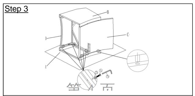
Attach Left Armrest (A) between Sofa Seat (D) and Sofa Back (C) using Bolts (1) and Washers (2) with Allen Key (3) as shown in Picture.
