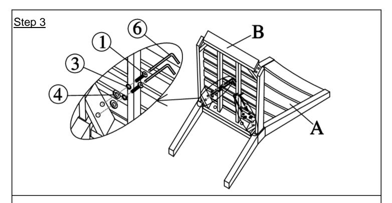
Attach Seat Panel(B) to Backrest Panel(A) using Bolts(1), Spring Washers(3), and Washers(4) with Allen Key(6).
