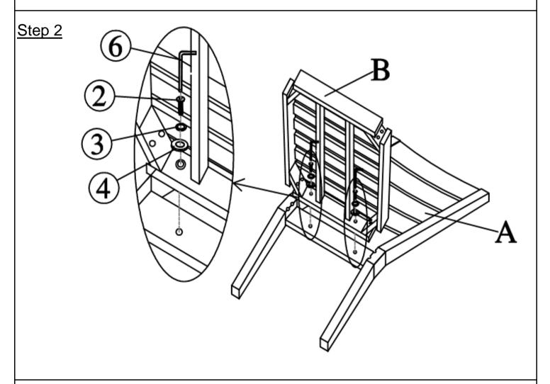
Place the Backrest Panel(A) facedown onto a clean, non-marring surface. Align Seat Panel(B) to Backrest Panel(A) then attach using Bolts(2), Spring Washers(3), and Washers(4) with Allen Key(6).
