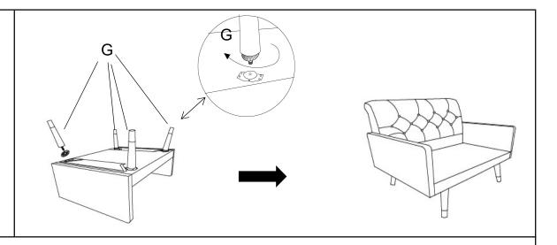
Install the Wood Legs with gasket(G) at the bottom of the Chair on the threaded stem. Then insert threaded stem into the mounting postion at the corner of the Chair. Tighten by turning the Leg clockwise.
