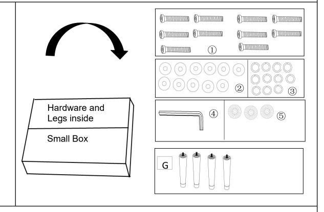
Open the Small Carton Box to take out the Wooden Legs(G), Gaskets(\$), Bolts(\$), Washers(\$), Spring Washers(\$), and Allen Key(\$).
