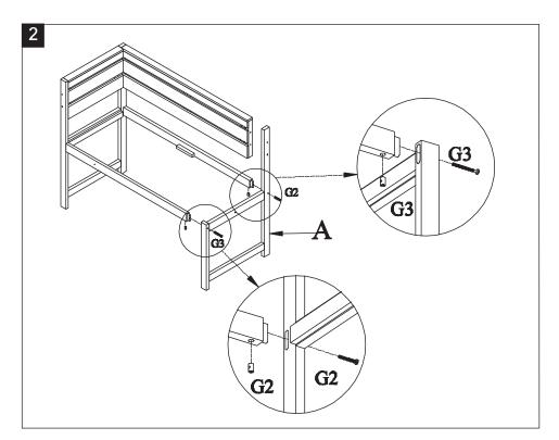
Step 2 : attach the leg(A) to the back (D),rear bar (E) and front bar (F) as shown on the picture. Then use the Allen bolt S (G2) to tighten the leg(A) to the rear bar (E) .Use the Allen bolt L (G3) to tighten the leg(A) to the front bar (F) as shown on the picture.
