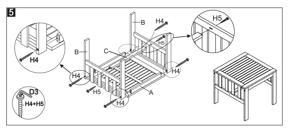
Step 5: attach the Table legs (F) and Support bar (G) to the Table top (E) as shown on the picture. Tighten each side by using the Allen screw L (H4) and Allen screw S (H5) with the Allen key (H7) as shown on the picture.
