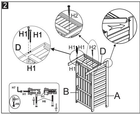
Step1: attach the Back(A) to the Seat (B) as shown on the the picture. Use the Allen screw (H2) tighten by using the Allen key (H7) as shown on the picture.
