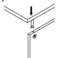
Insert the cam lock bolt into the pre-drilled hole above the cam connector.
