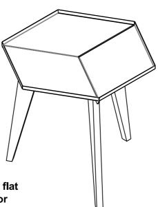
Make sure the unit is rested on a flat surface and does not feel loose or wobbly. If it does, double check all bolts/screws are secured and properly tightened.
