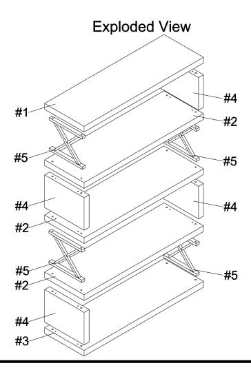
2) Align side frame (#5) to the holes of the top panel (#1),
