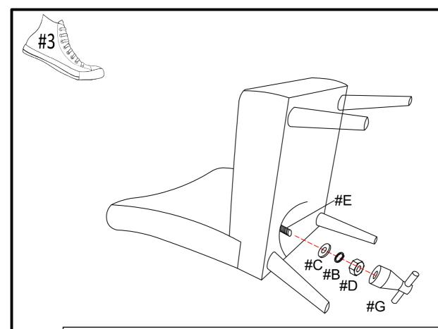
Open the compartment at the bottom of the seat (#1). Insert flat washer (#C) and lock washer (#B) to the threaded bolts (#E). Secure with hex nut (#D).
