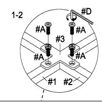
2. Insert 4 bolts (#A) into the the top holes and secure using the Allen wrench (#D).
