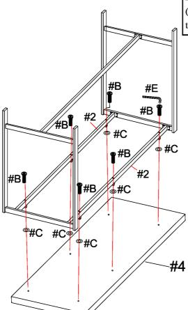
Prepare 6 bolts assembly by inserting washer (#C) onto bolts (#B). Align table base to the table top (#4), then secure by using bolts (#B).
