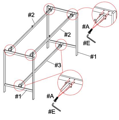
Align table leg supports (#2) and table leg bottom support (#3) to the holes of the table legs (#1).
