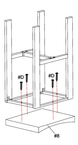
Align chair legs to the seat panel (#8), then secure by using screws (#D). There are no pre-drilled holes.
