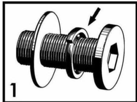
When lock or spring washer is used in an assembly, please make sure the lock or spring washer is placed between the larger flat washer and the head of the screw or bolt.
