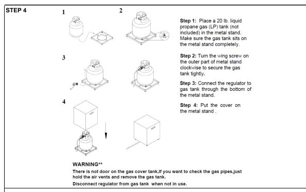
4. Place the 20lbs Propane Gas Tank (not included) into the Tank cover (09).
