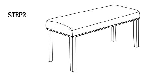
Do not tighten screws until completely assembled
