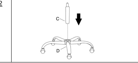
Insert the Gaslift(C) into the mounting position under of Chrome base(D) as pictured.
