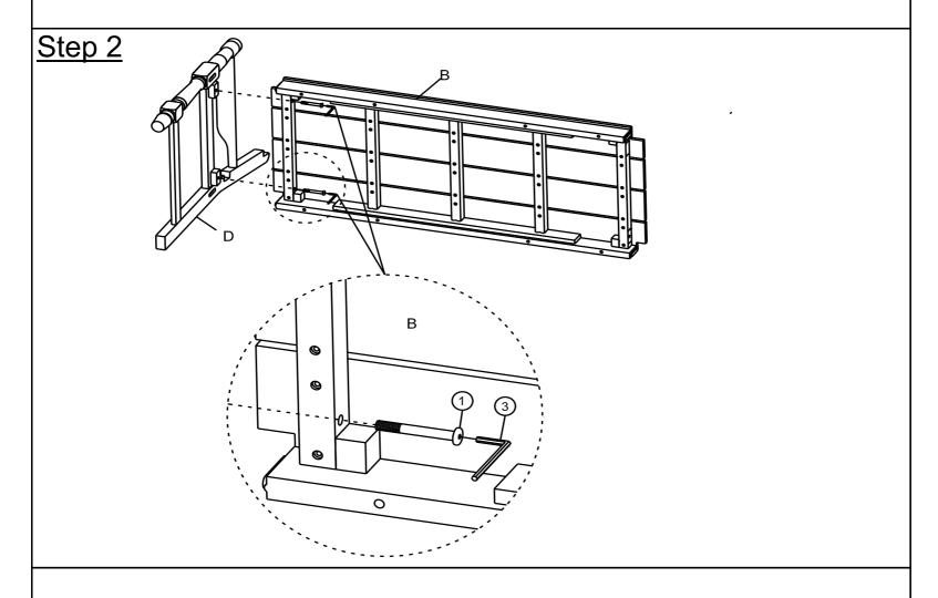
Insert the tenon of the Seat Panel(B) into the mortise of Left Leg(D) and Right Leg(E). Attach Left Leg(D) and Right Leg(E) to Seat Panel(B) using Bolts( $\widehat{1}$ ) with Allen Key( $\widehat{3}$ ) as shown above.
