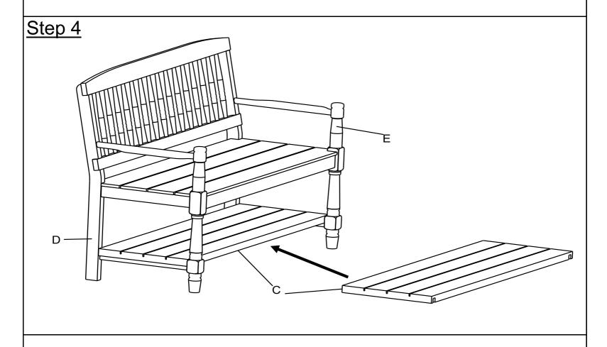
Insert Shelf(C) onto the bottom Rails of Left Leg(D) and Right Leg(E).
