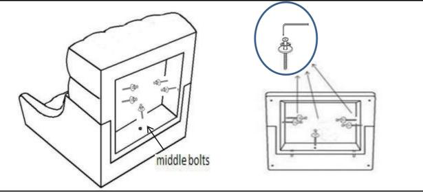
You should first fix the middle bolts on the Chair seat (B) tightly until there is no gap between Chair seat (B) and Chair backrest (A). Using hand to push Chair seat (B) forward a bit for finding and insert the bolts for sides correctly, and fix them.
