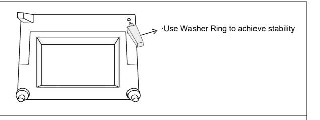
Install the leg into the chair by putting a Plastic Washer Ring(5) (improves tightness and security of leg)on the threaded stem.
