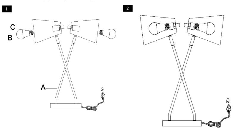
Step 1 Insert the bulb(B) into the socket(C).
