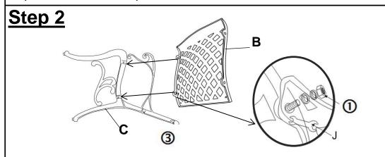
Attach the Chair Seat Panel(B) to the Left Legs with Left Legs with Pre-attached Levellers(C) using Washers, Spring Washers and Nuts((1)), with Spanner((3)). **DO NOT fully tighten at this stage.**
