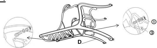
Repeat the same assembly process for the Right Legs with Arm and Preattached Bolts for Seat Panel and Leveller(D)
