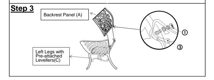
Then attach the Backrest Panel(A) to the top end of the Left Legs with Preattached Levellers(C)using Washers, Spring Washers and Nuts(1) with Spanner(3).
