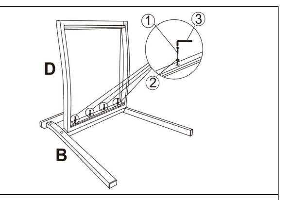
Open the carton and place all the parts onto a clean, non-marring surface. Attach Seat(D) to Right Armrest/Leg(B) using Bolts(1) And washer 2 with Allen Key(3) as shown above.
