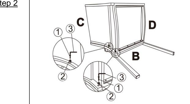
Attach Backrest(C) to Right Armrest/Leg(B) using Bolts(1) and Washer (2) with Allen Key(3)as shown above.
