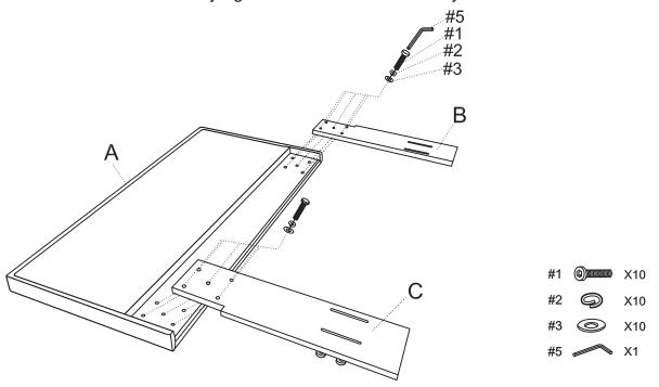
Step 2. Screw out the bolts on the headboard posts using allen wrench (part #5). Attach bed frame (\*Not Included) to left headboard post (part B) and right headboard post (part C) using bolts (part #1), spring washers (part #2), flat washers (part #3), nuts (part #4), allen wrench (part #5) and wrench (part #6).
