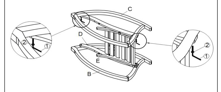
Attach Left Leg Panel(C) to Seat Panel(D) using Bolts(2) with Allen Key(1) as pictured above.
