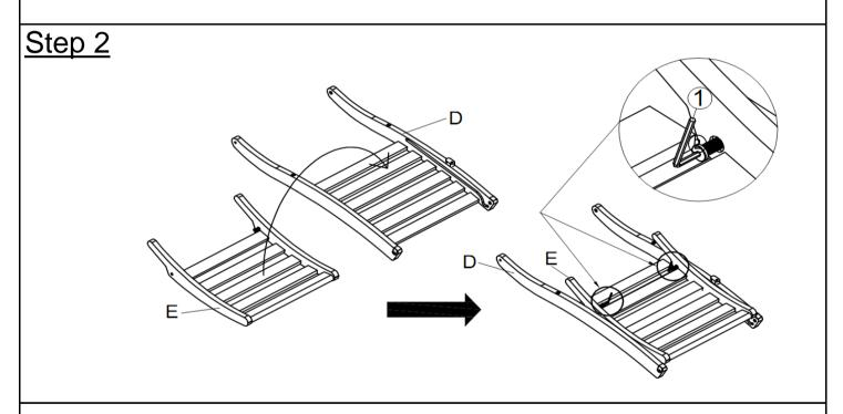
Align Footrest Panel(E) to Seat Panel(D) as pictured. Attach Footrest Panel(E) to Seat Panel(D) using Bolts(2) with Allen Key(1). **Do not fully tighten the Bolts.**
