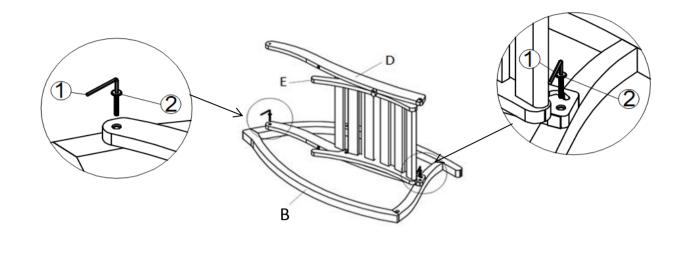
Attach Seat Panel(D) to Right Leg Panel(B) using Bolts(2) with Allen Key(1) as pictured above.
