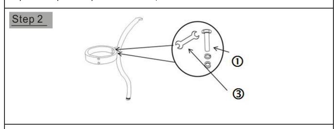
Loosely affix the Support Ring(C) to Table Leg with pre-attached Levellers (B) using Washers, Spring Washers, and Hex Bolts(1), with the Spanner(3).
