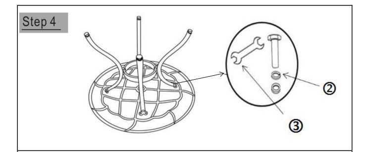
Lay the Table Top(A), facedown, onto a flat, soft, clean surface. Attach the Table Legs(B) to the Table Top(A) using Washers, Spring Washers, and Hex Bolts(2) with the Spanner(3).
