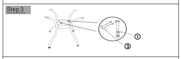
Repeat Step 2 to attach the remaining 3 Legs(B) to the Support Ring(C) **DO NOT OVERTIGHTEN**.
