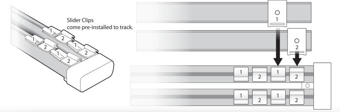
Adjust the panel track to the width needed. Be careful not to over extend the track and cause it to separate completely.
