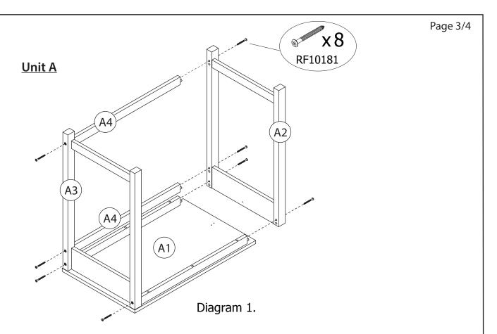
Step 1: Attach Top (A), Left Panel (A2), Right Panel (A3) and Crossbars (A4) together by using 8 Large screw (RF10181) as per diagram 1.
