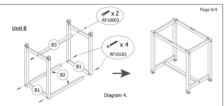
Step 4: Attach Side Panels (B1) into the Front and Back Crossbar (B2) by using 4 Large screw (RF10181) and Bottom Crossbar (B3) by using 2 Medium screw (RF10003) as per diagram 4.
