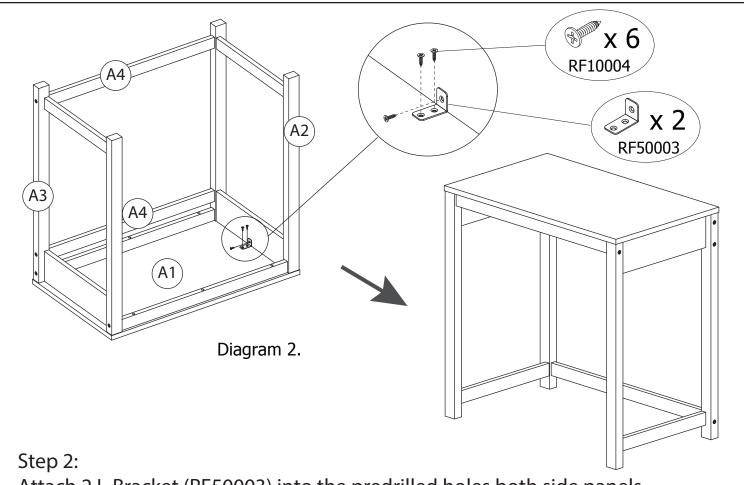
Attach 2 L-Bracket (RF50003) into the predrilled holes both side panels by using 6 Small screw (RF10004) as per diagram 2.
