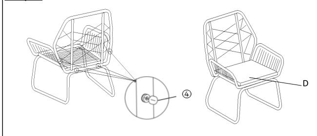
Put the PE Cap(4) on the bolts as the picture show above.
