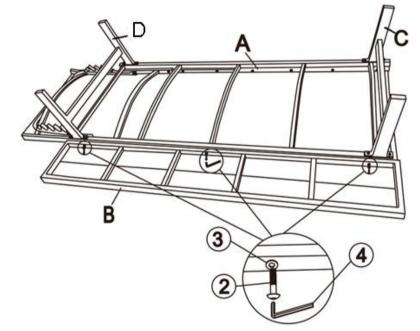
Attach Bench(B) to Seat Panel(A) using Bolts(2) and Washers(3) with Allen Key(4) as shown above.
