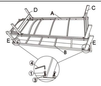
Attach the Bench Leg(E) to Bench(B) using Bolts(1) and Washers(3) with Allen Key(4) as shown above.
