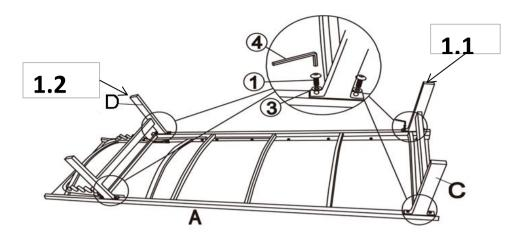
Open the carton and place all the parts onto a clean, non-marring surface. Place the Seat Panel(A) facedown.
