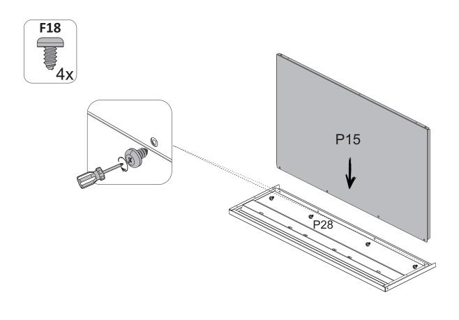
1 - Align parts **P12** and **P13** to part **P15**, until it leans against piece **P28**. 2 - Screw the two with **F18**. STEP 8
