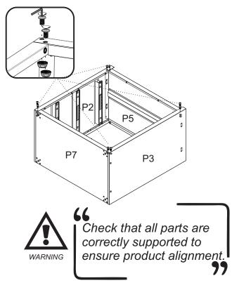
1 - Fit part P10 into parts P2, P3 and P5. Check that all fits are supported over the bolts. STEP 4
