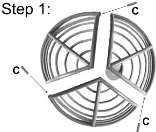
Insert dowels into pre-fitted holes in papasan bowl pieces
