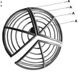
Join bowl piece with circular center part attached to another bowl piece using 4 of the longer bolts (Do not overtighten)
