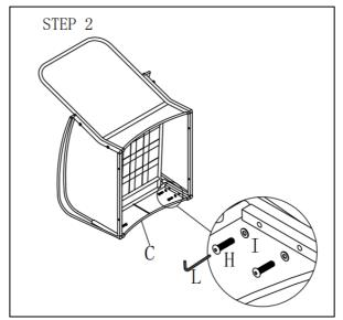
3. Locate the Chair Seat(C) to the Chair Back(D) by the pre-drilled threads. Fasten Bolts(H) with Washers A(I) by using Allen Key(L) to combine chair seat and chair back together. 2 bolts should be fastened totally. (Step 3).
