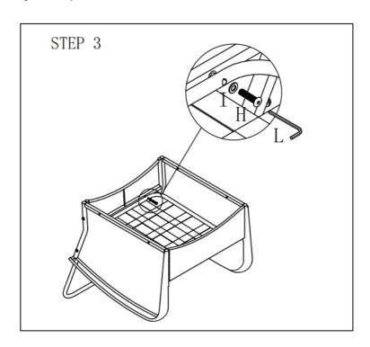
4. Locate the Rocking Track(E) to the Armrests' bottom(A & B) by the pre-drilled threads. Fasten Bolts(H) into Screw Nuts(K) by using Allen Key(L) and Hex Spanner(M) to combine rocking rack and the chair main part together. 4 bolts should be fastened totally. (Step 4).
