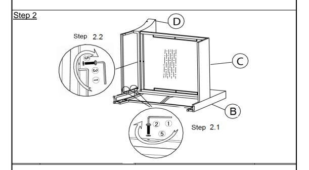
Step 2.1Attach Chair Back(D) to the Left Armrest(B) and Chair Seat(C) using Bolt(②) and Washer(⑤) with Allen Key(①). Step 2.2 Attach Chair Back(D) to the Left Armrest(B) and Chair Seat(C) using Bolt(③) and Washer(⑤) with Allen Key(①). Only loosely tighten the Bolts.
