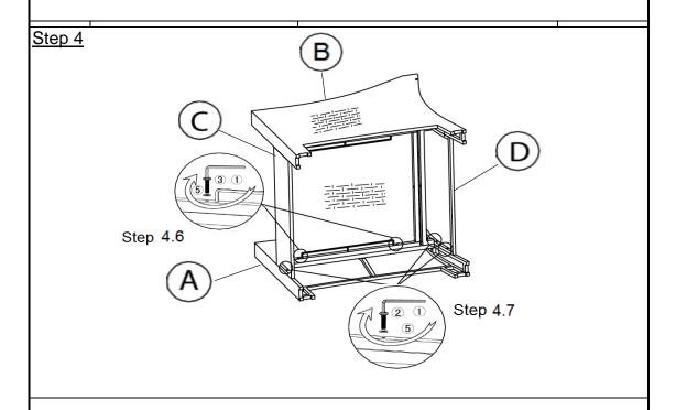
Step 4.6) Attach Right Armrest(A) to the Chair Seat(C) and Chair Back(D) using Bolt(③) and Washer(⑤) with Allen Key(④). Step 4.7) Attach Right Armrest(A) to the Chair Seat(C) and Chair Back(D) using Bolt(②) and Washer(⑤) with Allen Key(④). Only loosely tighten the Bolts.
