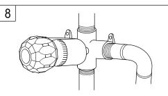
8. Turn on water supply and check connections for leaks. Place handle on valve stem and flush lines by running hot and cold water uninterrupted for one minute.
