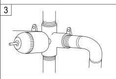
3. Connect water supply lines to valve. (Hot water to left and cold water to right side of valve.) Use compound or tape on all threaded connections. Connect valves to spout.
