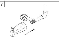
7. Apply pipe compound to tub spout nipple and attach spout to nipple. Hand tighten.
