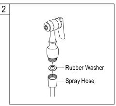
2. Place rubber washer to end of spray hose and attach sprayer.
