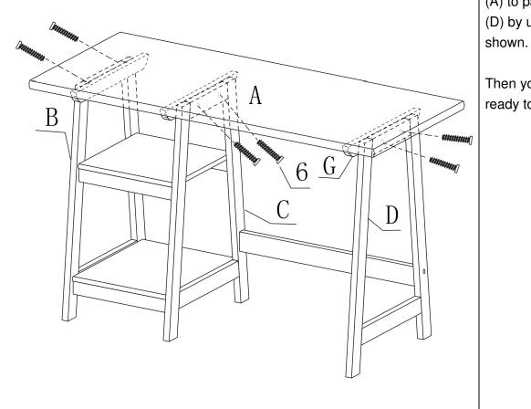
Step 8: Attach wood top (A) to panels (B),(C), (D) by using bolt (6) as
