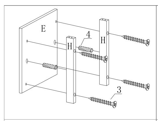
Step 3: Attach short stretcher (H) to bottom shelf (E) by using screw (3) and dowel (4) as shown.
