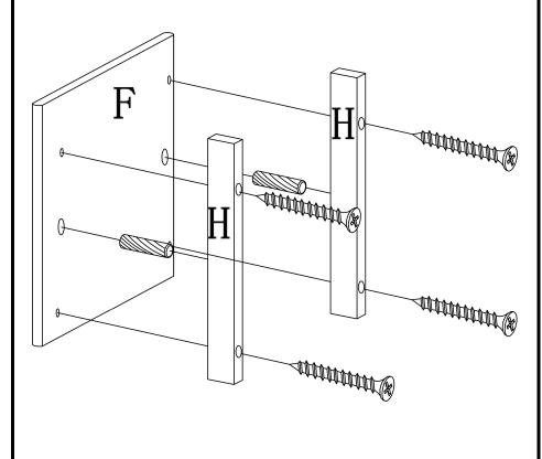
Step 2: Attach short stretcher (H) to top shelf (F) by using screw (3) and dowel (4) as shown.
