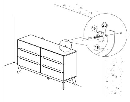
5. Finally, attach safety strap (16) and washer (17) using 4x30mm screw (15) to the wall.
