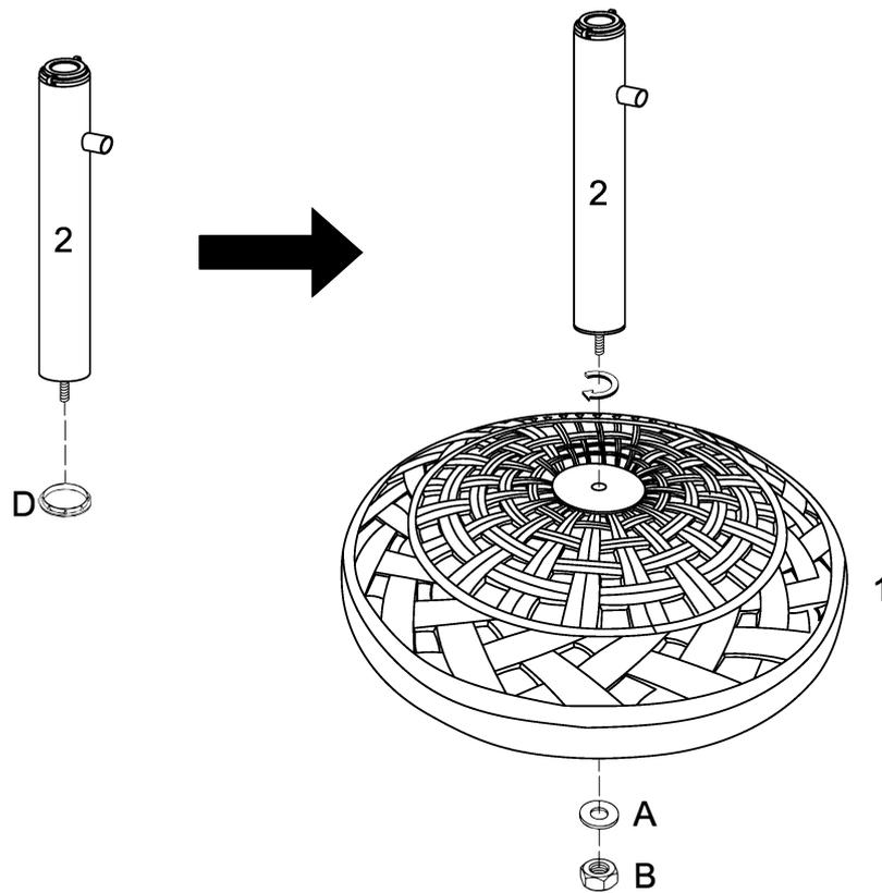
Put plastic cap (D) in the bottom of the Metal Tube (2) to the Center Hole of the Round Base (1), and secure it with the Washer (A) and Nut (B).
