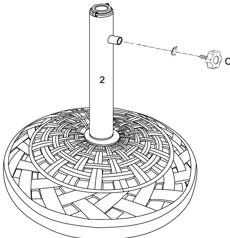
Twist the Knob (C) to the Metal Tube (2) as per diagram.
