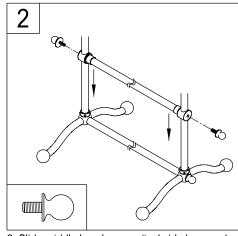
2. Slide middle bar down vertical side bars and tighten bolts at desired level.
