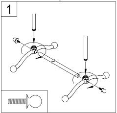
Screw in 29" vertical side bars into foot and bolt in bottom bar between assembly.
