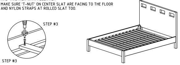
PLACE SLAT ASSEMBLY INTO BED ASSEMBLY AND DRILLING 14 PCS PHILLIPS HEAD WOOD SCREWS INTO EVERY OTHER SLAT FOR FITTING
