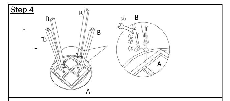
Repeat step 3, attaching the remaining 3 legs to the Table Top(A). Then proceed to tighen all Bolts at all joints in a sequential manner.
