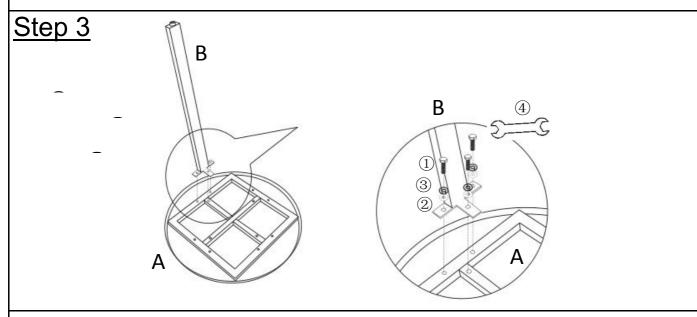
Align the mounting positions on Table leg(B) and Table Top(A). Attach Leg(B) to Table Top(A) using Washer(2), Spring Washer(3) and Bolt(1) with Spanner (4).
