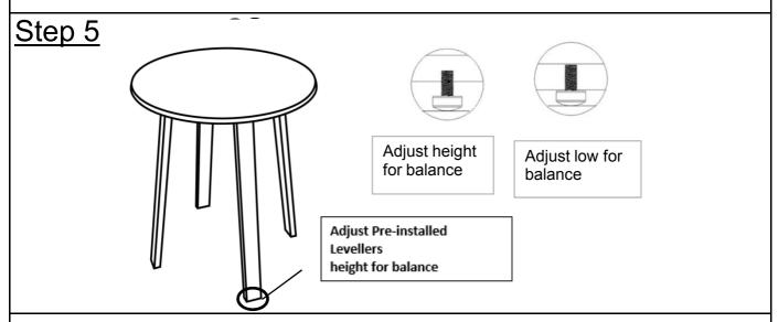
Adjust the Pre-installed Levellers at the base of the Legs until the Table is level with the ground.
