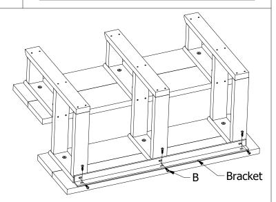
2) Attach the metal bracket to the bottom of the top tread as shown using B screws. The tread contains pilot holes to help align the bracket. (6) screws are used for the 32" step and (8) on the 48" step.
