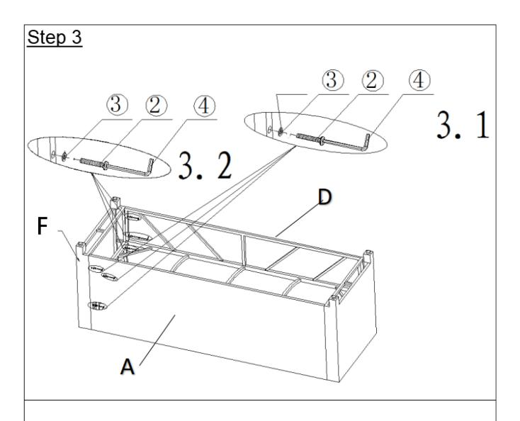
Insert the positioning dowels on Backrest(A) into Left Armrest(F).
