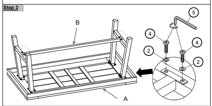
Attach the Support Bar (B) to the Legs as shown in picture above. Affix the Support bar (B) with the Legs by using Small bolts (2), Small washer (4) and Allen key (5), Total 4 posittions.
