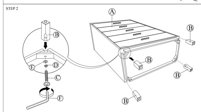
Insert Leg (B) at position as shown and tighten with JCBC Screw (C), Spring Washer (D) & Flat Washer (E) by using Allen key (F)  $\,$
